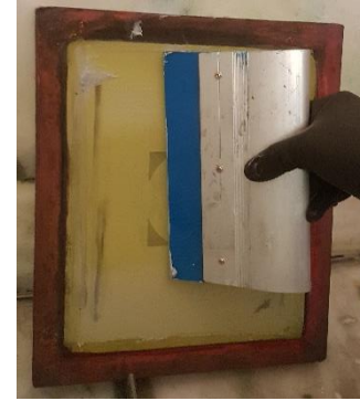
Apply SISS Super Stain to the screen using a spatula / palette knife or Squeegee
