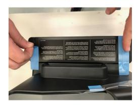
Unclip the ink tank on the right hand side of the printer and remove blue tape
