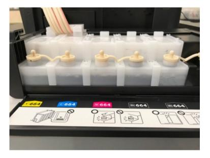
Re-clip ink tank back onto the side of the printer
